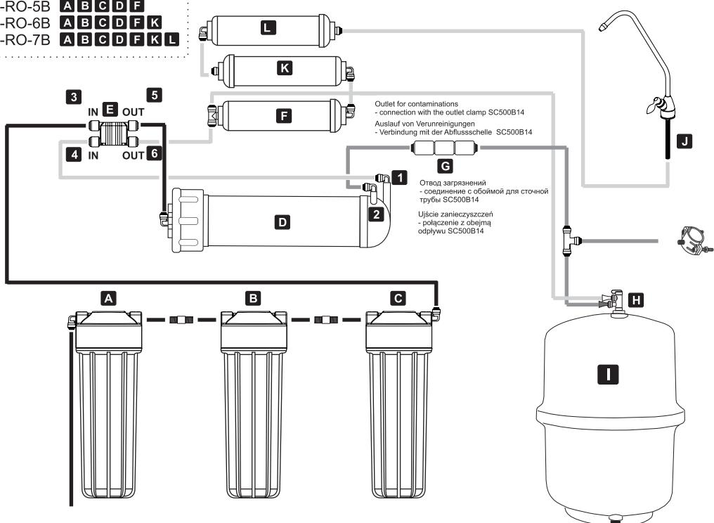
Water supply to the filter from the FT06 or FT07, FT03 connection (option)
